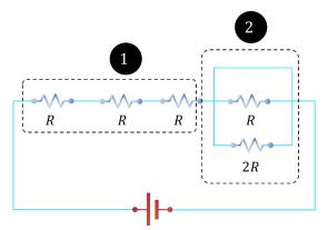
In  $2^{nd}$  part of diagram a connecting wire is nullifying the resistance of parallel resistance thus their new resistance is zero. So, net resistance of circuit is 3R
