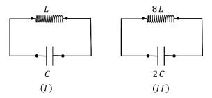
Then find  $\omega_1/\omega_2$ , where  $\omega_1$  and  $\omega_2$  are resonance frequencies of the two circuits.
